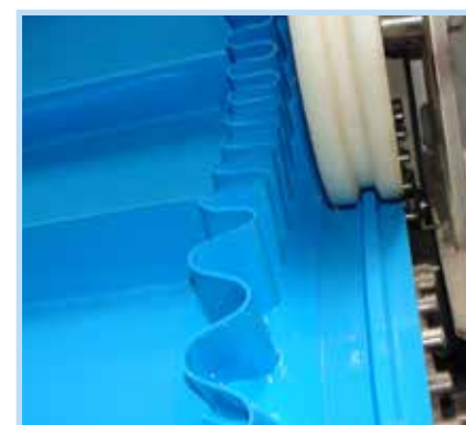
3. Two parallel guides on the top side of the belt used in elevators to maintain belt rigidity.
